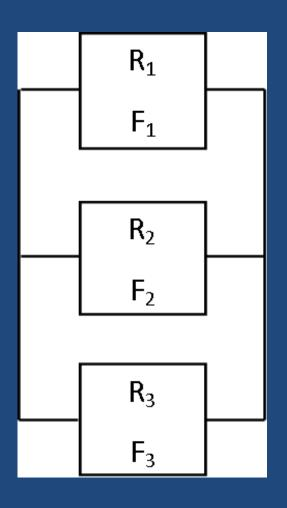
$$R_{S}(t) = R_{1}R_{2}R_{3} + R_{1}R_{2}F_{3} + R_{1}F_{2}R_{3} + F_{1}R_{2}R_{3} + R_{1}R_{2}R_{3} = R_{1}R_{2}R_{3} + R_{1}R_{2}(1 - R_{3}) + F_{1}(1 - R_{2})R_{3} + (1 - R_{1})R_{2}R_{3} = R_{1}R_{2} + R_{1}R_{3} + R_{2}R_{3} - 2R_{1}R_{2}R_{3}$$
