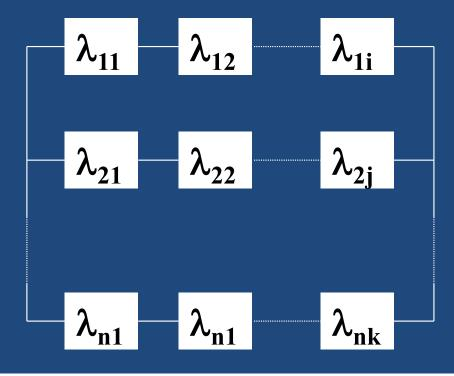
$$R_{S}(t) = 1 - \left[ \left( 1 - \prod_{i=1}^{i} R_{1i} \right) \left( 1 - \prod_{j=1}^{j} R_{2j} \right) \dots \left( 1 - \prod_{k=1}^{k} R_{nk} \right) \right]$$
