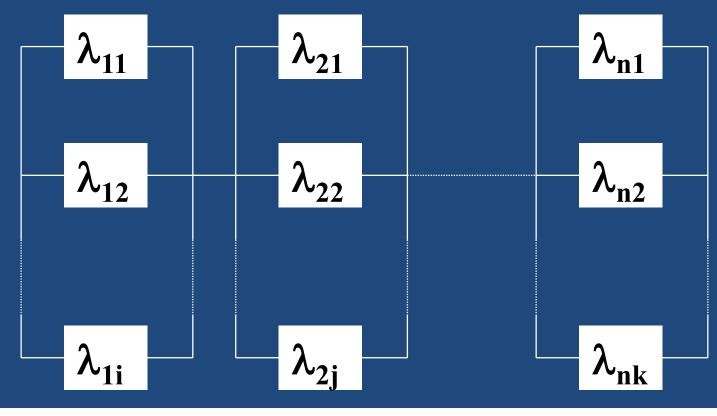
$$R_{S}(t) = \left[1 - \prod_{1=1}^{i} (1 - R_{1i})\right] \left[1 - \prod_{j=1}^{j} (1 - R_{2j})\right] \dots \left[1 - \prod_{k=1}^{k} (1 - R_{nk})\right]$$
